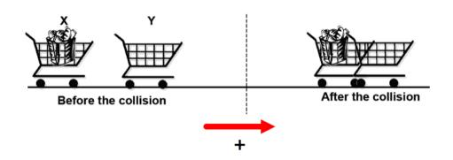
Notice how the direction that we consider positive is marked with an arrow and a "plus" sign? This is the original direction of Trolley X.
