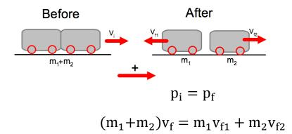
Here, one object exploded and seperated so there was one object before and two objects after. So the final equation has three pieces.
