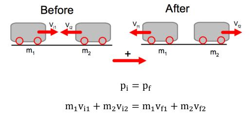
Notice how each separate object has its own "mv". Here, two objects collided and left seperately so there were two objects before and two objects after. So the final equation has four pieces.
